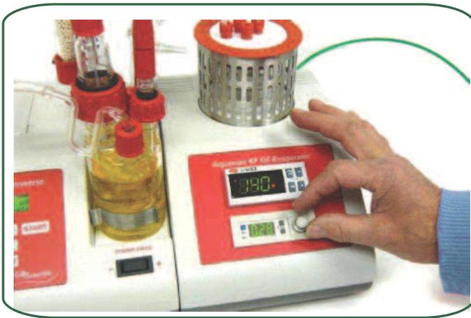
Adjusting carrier gas flow.
