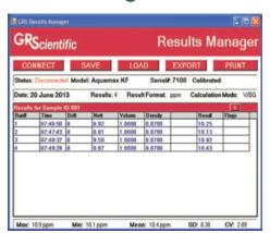
This is a windows application that allows you to view and print sets of results created by the Aquamax KF Coulometric. It can download results directly from the titrator through a serial port connection, or open result files previously
