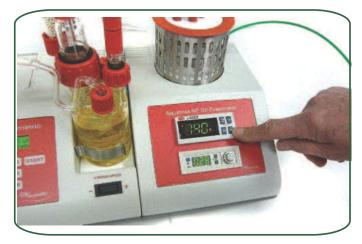
Adjusting carrier gas flow.
