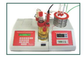
The oven temperature can be adjusted from ambient to 200°C and a digital carrier gas flow setting of 300 ml per minute.
